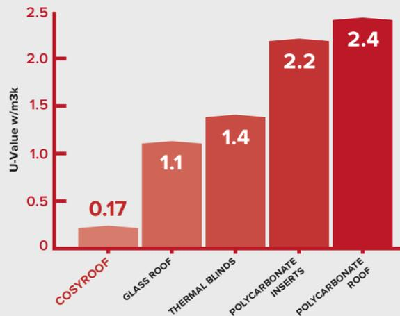
U value measures how well a building component heats the inside of a structure. The lower the U value, the less heat is lost.
